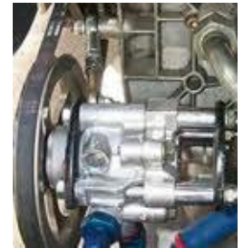
New power steering pump installed
