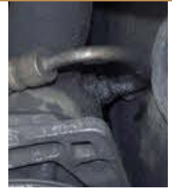
Power steering leak at pump
