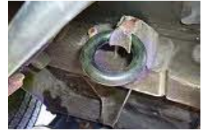
New exhaust hanger, ready to be attached
