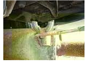
Broken exhaust hanger
