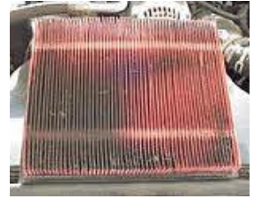
Dirty and restricted air filter
