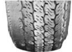
Signs of irregular tire wear
