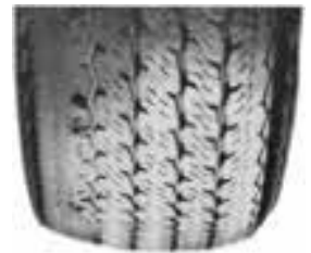
Irregular wear due to tire imbalance
