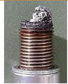
Worn out spark plug
