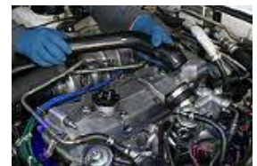
Removing a valve cover to replace gasket
