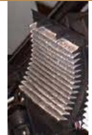
A dirty and clogged cabin air filter
