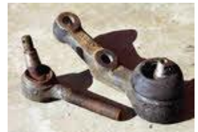
Worn out ball joint and tie-rod end
