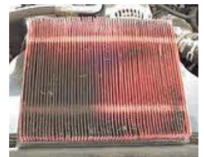
Dirty and restricted air filter
