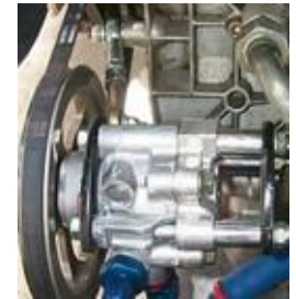
New Power Steering Pump Installed
