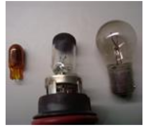
Examples of Burned Out Bulbs
