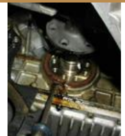
Removing a Leaking Rear Main Seal.
