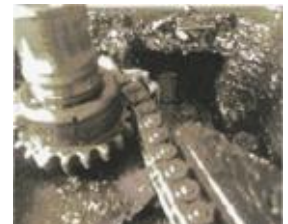
Sludge From Lack of Oil Changes
