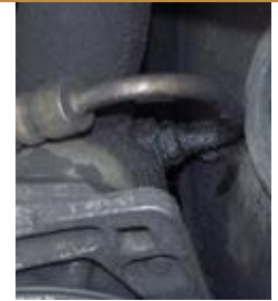
Power Steering Leak at Pump
