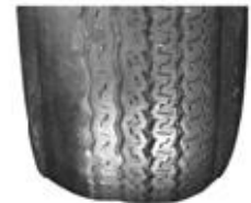
Worn out struts damage tires.
