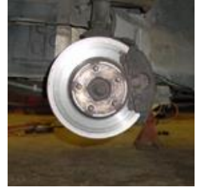
Damaged Brake Rotor (metal to metal contact)
