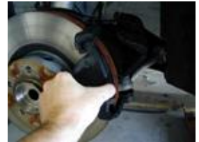
Installing New Brake Pads
