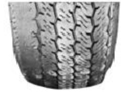
Signs of irregular tire wear.
