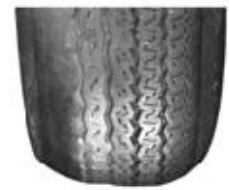
Worn out struts damage tires.
