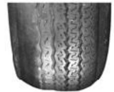
Worn out struts damage tires.
