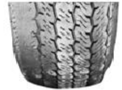
Signs of irregular tire wear.
