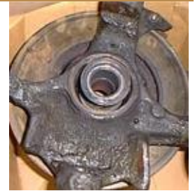
Wheel Bearing Failure; Seized.
