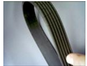
Cracked/Worn Accessory Drive Belt
