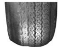
Worn out struts damage tires.
