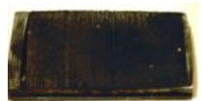
Extremely Dirty/Restricted Air Filter
