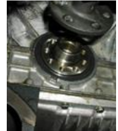
New Rear Main Seal Installed on Engine.
