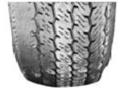
Signs of irregular tire wear.
