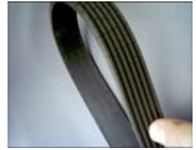
Cracked/Worn Accessory Drive Belt
