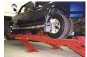
A Wheel alignment being Performed.
