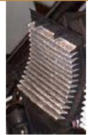
A dirty and clogged cabin air filter
