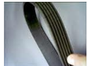
Worn accessory drive belt
