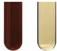
Brake fluid before and after service
