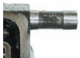
Valve body spool with heavy build up
