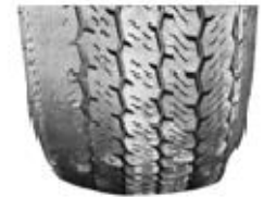
Signs of irregular tire wear.
