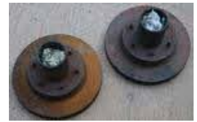
Worn or damaged rotors needing resurfacing
