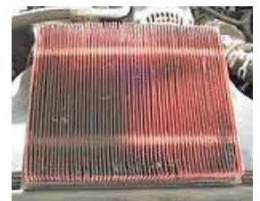
Dirty and restricted air filter
