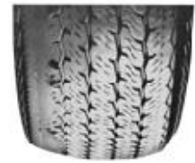
Irregular wear due to tire imbalance.
