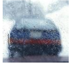
Impaired View From Worn Wiper Blades
