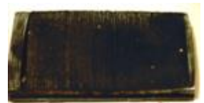
Extremely Dirty/Restricted Air Filter
