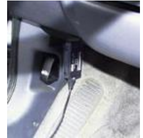
Scanning vehicle for trouble codes.
