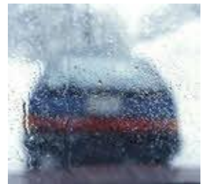
Impaired view from worn wiper blades
