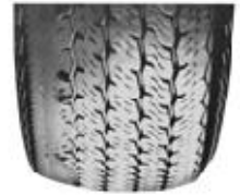
Irregular wear due to tire imbalance.
