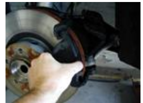
Installing New Brake Pads
