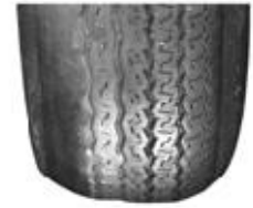
Abnormal tire wear from bad alignment
