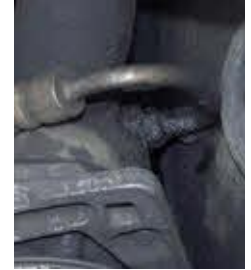
Power steering leak at pump
