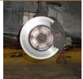
Damaged brake rotor from metal-to-metal contact
