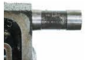
Valve body spool with heavy build up
