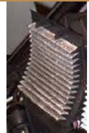
A dirty and clogged cabin air filter
