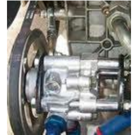
New power steering pump installed
