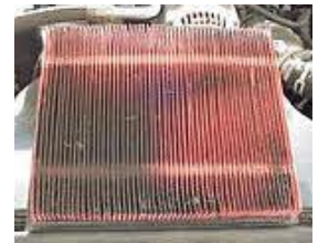
Dirty and restricted air filter
