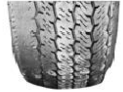
Uneven tire wear due to worn shock absorbers.
