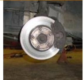
Damaged Brake Rotor (metal to metal contact)
