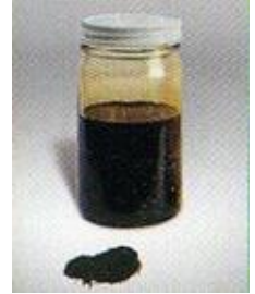
Dirty, worn power steering fluid.
