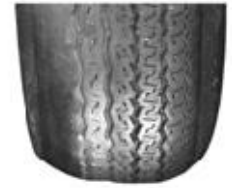
Abnormal Tire wear From a Vehicle that is out of Alignment.
