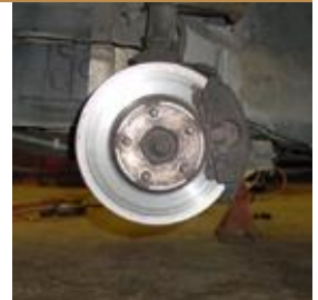
Damaged brake rotor from metal-to-metal contact
