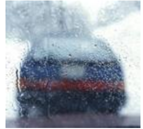
Impaired view from worn wiper blades
