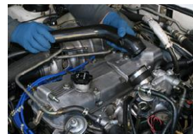
Removing a valve cover to replace gasket
