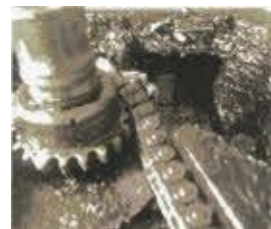
Sludge from lack of oil changes
