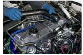
Removing a valve cover to replace gasket
