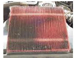
Dirty and restricted air filter
