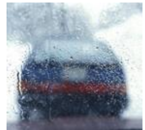
Impaired View From Worn Wiper Blades
