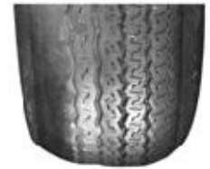
Worn out struts damage tires.
