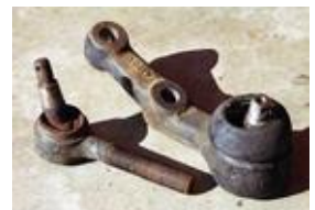
Worn Out Ball Joint and Tie Rod End
