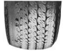
Irregular wear due to tire imbalance.
