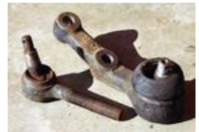
Worn Out Suspension/Steering components.
