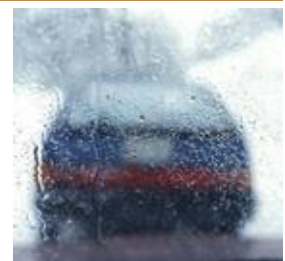
Impaired View From Worn Wiper Blades
