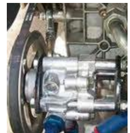
New power steering pump installed
