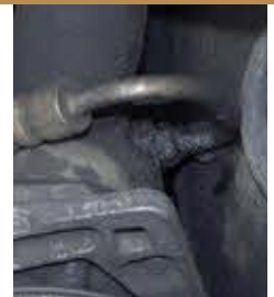
Power steering leak at pump
