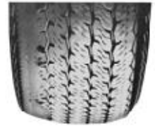
Irregular wear due to tire imbalance
