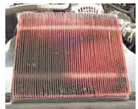
Dirty and restricted air filter
