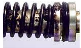
Harmful deposits on brake master cylinder piston assembly
