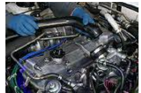
Removing a valve cover to replace gasket
