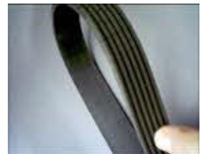
Worn accessory drive belt
