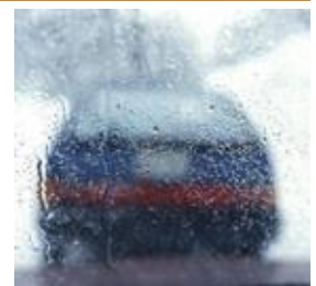
Impaired View From Worn Wiper Blades
