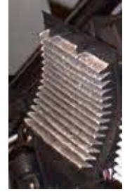
A dirty and clogged cabin air filter
