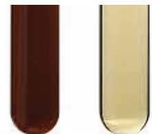
Brake fluid before and after service
