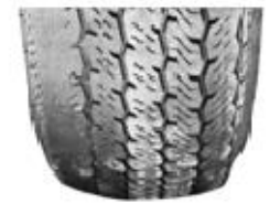
Signs of irregular tire wear
