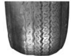
Abnormal tire wear from bad alignment
