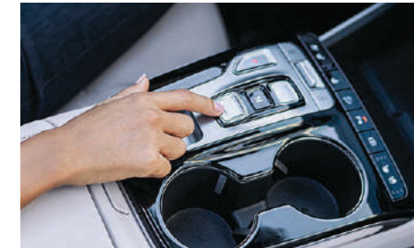
Electronic push-button gear selection
