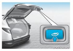
Press the power liftgate inner button for approximately one second when the liftgate is opened.
