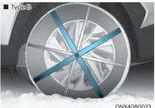
Since the sidewalls of radial tires are thinner than other types of tires, they may be damaged by mounting some types of tire chains on them. Therefore, the use of snow tires is recommended instead of tire chains. If tire chains must be used, use genuine HYUNDAI parts if available and install the tire chain after reviewing the instructions provided with the tire chains. Damage to your vehicle caused by improper tire chain use is not covered by your vehicle manufacturer's warranty.
