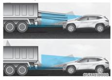
If the vehicle in front of you has cargo that extends rearward from the cab, or when the vehicle in front of you has higher ground clearance, additional special attention is required. Forward Collision-Avoidance Assist may not be able to detect the cargo extending from the vehicle. In these instances, you must maintain a safe braking distance from the rearmost object, and if necessary, steer the vehicle and depress the brake pedal to reduce your driving speed in order to maintain distance.
