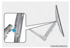
4. Install the new blade assembly by inserting the center part into the slot in the wiper arm until it clicks into place.
