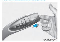
In the OFF (O) position, pull the lever gently toward you to spray washer fluid on the windshield and to run the wipers 1-3 cycles. The spray and wiper operation will continue until you release the lever. If the washer does not work, you may need to add washer fluid to the washer fluid reservoir.
