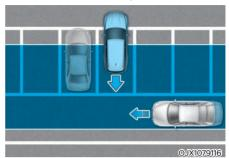
Rear Cross-Traffic Safety system may detect vehicles passing by behind you when parking in reverse into a parking space. If this occurs, the function may unnecessarily warn the driver and control the brake.
