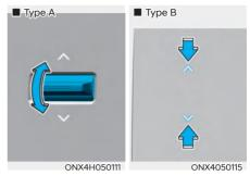
The temperature setting will increase when you toggle up or touch the UP arrow on the touchscreen (if equipped).
