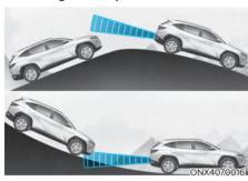
Blind-Spot Safety system may not operate properly when driving on a slope. The function may not detect the vehicle in the next lane or may incorrectly detect the ground or structure.
