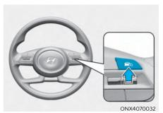
To turn off the Smart Cruise Control Press the Driving Assist button to turn Smart Cruise Control system off.
