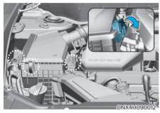
1. Loosen the air cleaner cover attaching clips and open the cover.
