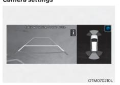
You can change Rear View Monitor 'Display Contents' or 'Display Settings' by touching the setup icon (♠) on the screen while Rear View Monitor is operating, or selecting 'Driver assistance → Parking safety → Camera settings' from the Settings menu while the engine is on.
