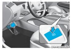
To release EPB (Electronic Parking Brake):
