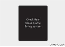
When Rear Cross-Traffic Safety system is not working properly, the 'Check rear cross-traffic safety systems' warning message will appear on the cluster, and the function will turn off automatically or the function will be limited. Have the vehicle inspected by an authorized HYUNDAI dealer.
