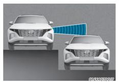
Blind-Spot Safety system may not operate properly when driving where the heights of the lanes are different. The function may not detect the vehicle on a road with different lane heights (underpass joining section, grade separated intersections, etc.).
