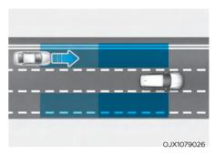
Blind-Spot Collision-Avoidance Assist helps detect and informs the driver that a vehicle is approaching at high speed from the blind spot area.
