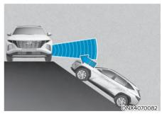
Rear Cross-Traffic Safety system may be limited when the vehicle is on a uphill or downhill slope, or near it, and may not detect the vehicle approaching from the left or right. If this occurs, the function may not warn the driver or control the brakes when necessary.
