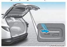
Your vehicle is equipped with the emergency tailgate safety release lever located on the bottom of the tailgate inside the vehicle.
