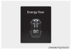
The engine braking is simultaneously used to decelerate the vehicle and to charge up the high-voltage battery.
