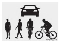
The illustration above shows the image the front view camera will detect as a vehicle, pedestrian and cyclist.
