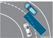
Blind-Spot Safety system may not operate properly when driving on a curved road. The function may not detect the vehicle in the next lane.
