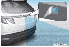
The rear view camera is used as a detecting sensor to help detect pedestrians. If the camera lens is covered with foreign material, such as snow or rain, it may adversely affect camera performance and Reverse Parking Collision-Avoidance Assist may not operate normally. Always keep the camera lens clean.
