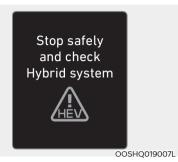
This message is displayed when there is a problem with the hybrid control system. The "\(\frac{1}{42}\)" indicator will blink and a warning chime will sound for approximately 10 seconds until the problem is solved. Refrain from driving when the warning message is displayed.
