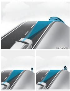
Forward Collision-Avoidance Assist may not detect the vehicle, pedestrian or cyclist in front of you while driving uphill or downhill adversely affecting the performance of the sensors.
