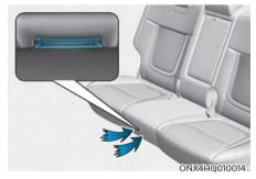
The hybrid battery cooling duct is located of the Passenger's seat. The cooling duct cools down the hybrid battery. When the hybrid battery cooling duct is blocked, the hybrid battery may be overheated.
