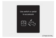
In traffic, your vehicle will stop if the vehicle ahead of you stops. Also, if the vehicle ahead of you starts moving, your vehicle will start as well. In addition, after the vehicle has stopped and a certain time have passed, the 'Use switch or pedal to accelerate' message will appear on the cluster. Depress the accelerator pedal or push the + switch, - switch or IID switch to start driving.
