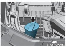
Check the fluid level in the washer fluid reservoir and add fluid if necessary. Plain water may be used during summer months if washer fluid is not available. However, use washer solvent with antifreeze characteristics in cold climates to prevent freezing.
