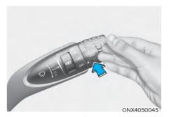
Push the lever away from you to spray rear washer fluid and to run the rear wipers 1~3 cycles. The spray and wiper operation will continue until you release the lever.
