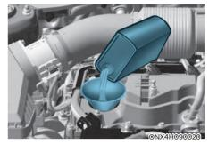
Check if the oil level is between the F-L line and refill it if the oil level is below the L, add enough oil to bring the level to F.
