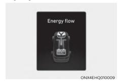
The engine charges up the high-voltage battery. The motor power is used to drive the vehicle.
