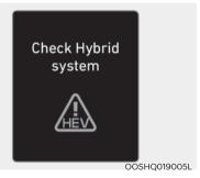
This message is displayed when there is a problem with the hybrid control system. Refrain from driving when the warning message is displayed.
