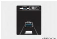
If you want to speed up temporarily without altering the set speed while Smart Cruise Control is operating, depress the accelerator pedal. While the accelerator pedal is depressed, the set speed, distance level and target distance will blink on the cluster.
