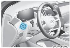
Detach the speed restriction label (1) from the sealant bottle (2), and place it in a highly visible place inside the vehicle such as on the steering wheel to remind the driver not to drive too fast.
