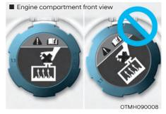
Check if the coolant cap label is straight in front.
