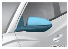
Your vehicle is equipped with both lefthand and right-hand Side view mirrors. The mirrors can be adjusted remotely with the mirror adjustment control switch. The side view mirrors can be folded manually to help prevent damage when going through an automatic car wash or when passing through a narrow street.
