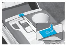
Downhill Brake Control assists the driver to descend down a steep hill without having to depress the brake pedal.
