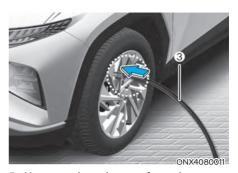
5. Unscrew the valve cap from the valve of the defective and screw the connection hose (3) of the compressor and tire.
