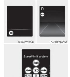
Displaying speed limit Speed limit information is displayed on the instrument cluster.
