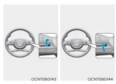
To resume Manual Speed Limit Assist after the function was paused, push the +, -, || 5 switch.
