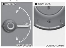
This gauge indicates the approximate amount of fuel remaining in the fuel tank.
