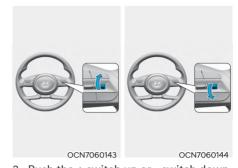
Push the + switch up or - switch down, and release it at the desired speed.
