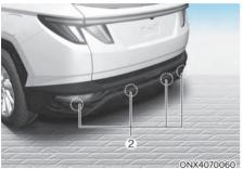
[1]: Rear view camera,[2]: Rear ultrasonic sensors
