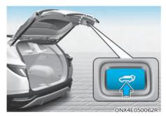
Press the power liftgate open/close button located inside the liftgate for more than 3 seconds. Close the liftgate manually after hearing the buzzer sound. The liftgate will open to the automatically adjusted height that was set.
