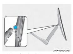
3. Lift up the wiper blade, and pull it out.
