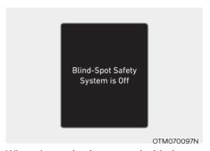
When the engine is restarted with the function off, the 'Blind-spot safety system is Off' message will appear on the cluster.
