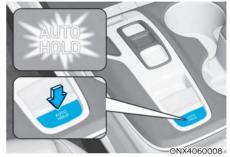
With the driver's door, engine hood and liftgate closed, then press the [AUTO HOLD] switch. The white AUTO HOLD indicator will come on and the system will be in the standby position.
