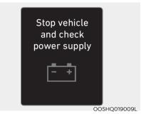
This message is displayed when a failure occurs in the power supply system.
