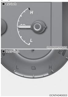
This gauge indicates the remaining hybrid battery power. If the SOC is near the "L (Low)" level, the vehicle automatically operates the engine to charge the battery.
