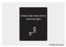
When the side view mirror warning light is not working properly, the 'Check side view mirror warning light' warning message will appear on the cluster. Have the vehicle inspected by an authorized HYUNDAI dealer.
