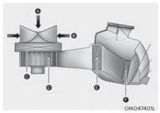
[A]: Outside air, [B]: Recirculated air [C]: Cabin air filter, [D]: Blower
