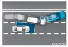
When changing lanes by detecting the lane ahead, if Blind-Spot Collision-Avoidance Assist judges that there is a collision risk with an approaching vehicle in the blind spot, it will help avoid a collision by applying the brake.
