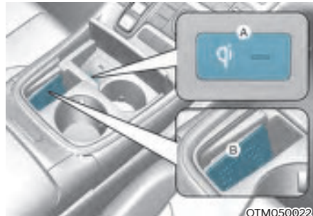
[A] : Indicator light [B] : Wireless Charging Pad (In-vehicle Authentication Pad)
