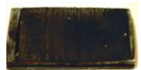
Extremely Dirty/Restricted Air Filter
