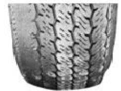
Signs of irregular tire wear.
