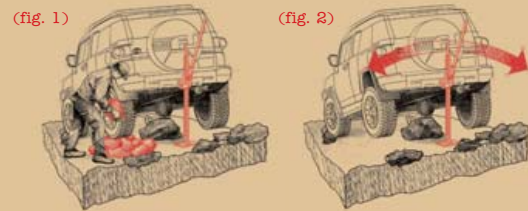
Fig. 1: Before jacking, make sure you have a proper jack point and solid footing. Once the vehicle has been elevated clear of the obstruction, place rocks or fallen branches under the tires for traction or for needed height, then lower the vehicle and drive off. Fig. 2: Another option is to "pole-vault" the elevated vehicle by pushing it off the jack onto solid ground.
