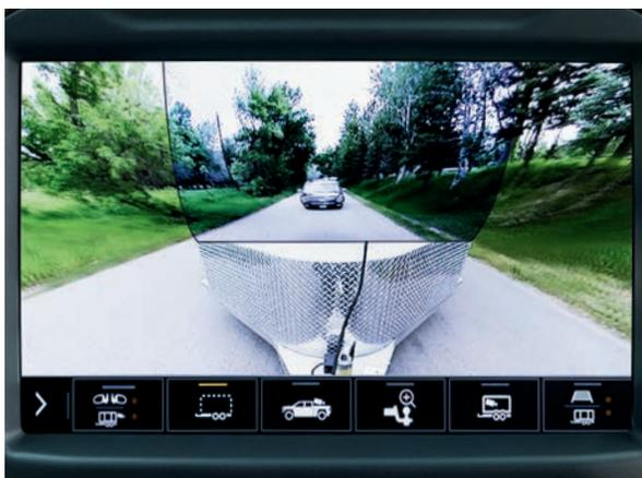
**Transparent Trailer** Allows the driver to virtually “see through” a conventional hitched box or camping trailer.
