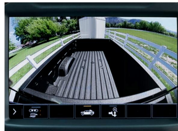
**Bed View** Allows you to see inside the cargo bed to help with fifth-wheel or gooseneck hitching and to check on cargo.
