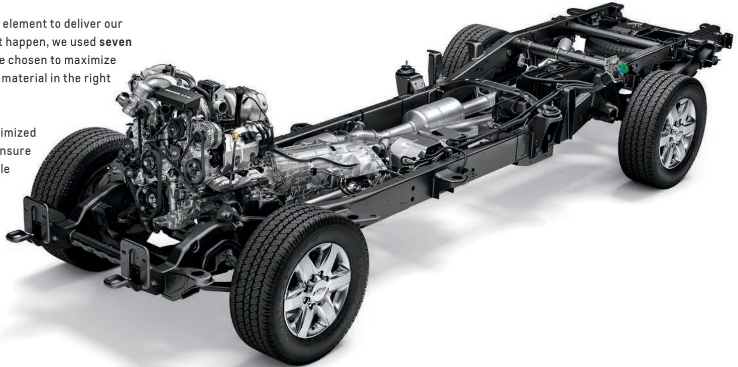
The chassis is **20% stiffer** than the previous generation. To achieve that target, we used a combination of high-strength and ultra-high-strength steel throughout the cab and frame.
