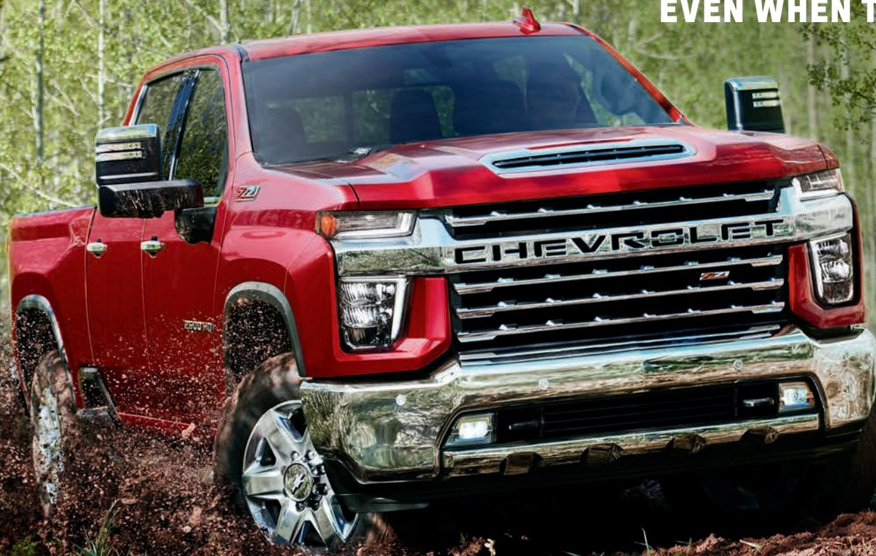
The available **Z71 Off-Road Package** provides legendary capability and includes all-terrain tires, an off-road tuned suspension featuring twin-tube shocks, an underbody skid plate package and Hill Descent Control.
