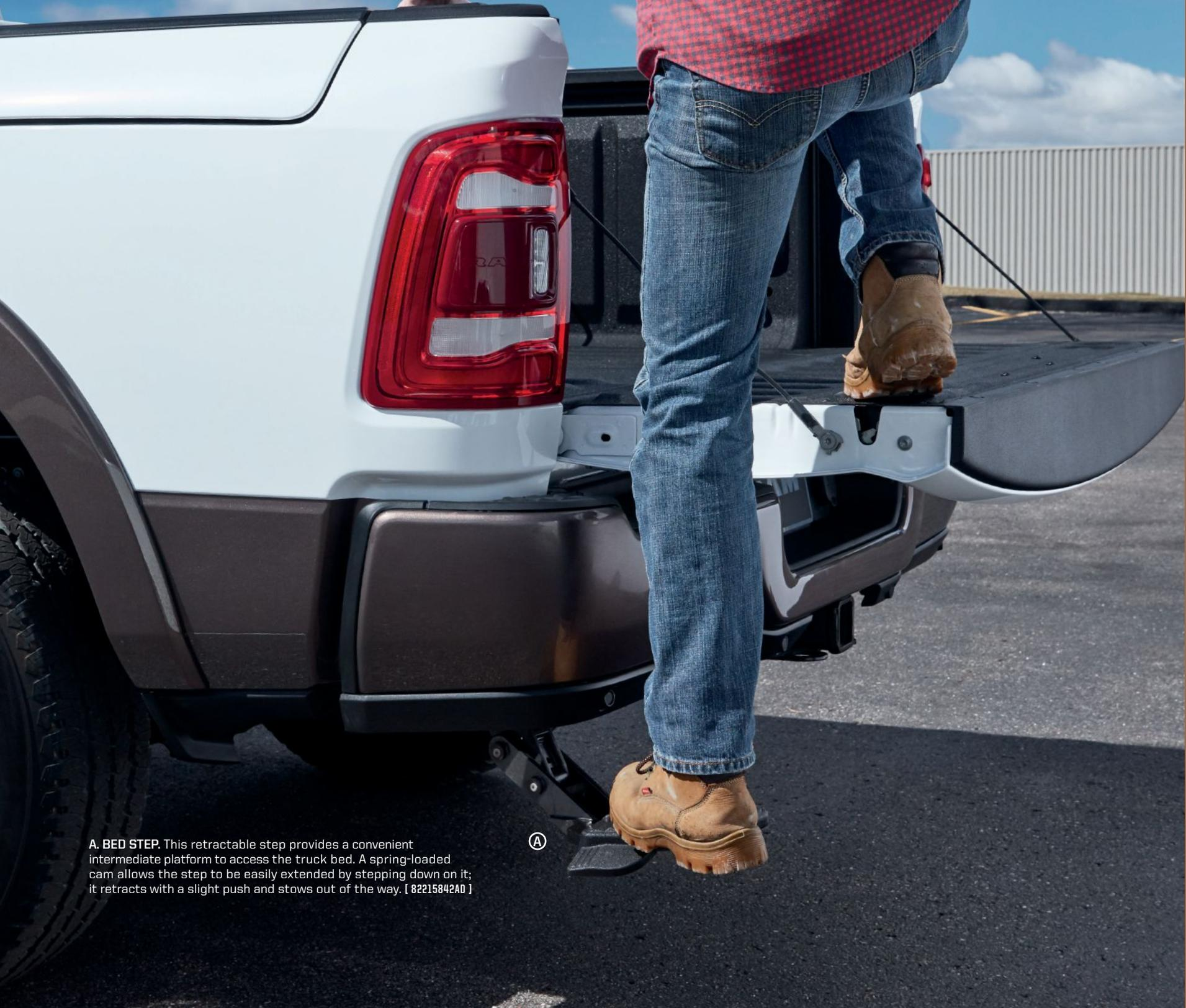
**A. BED STEP.** This retractable step provides a convenient intermediate platform to access the truck bed. A spring-loaded cam allows the step to be easily extended by stepping down on it; it retracts with a slight push and stows out of the way. [ 82215842AD ]
