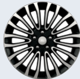
18" Machined Face Aluminum with Painted Pockets Standard: Titanium, Titanium Hybrid, Platinum Hybrid Available: SE, SE Hybrid Optional: Fusion Energi SE, Fusion Energi Titanium, and Fusion Energi Platinum
