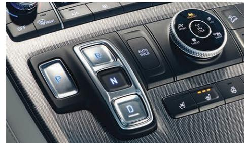
Shift-by-Wire push-button gear selection
