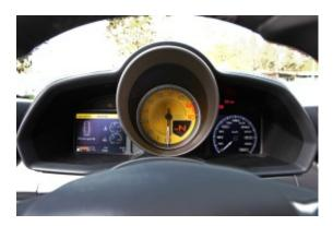
The instrument cluster consists of a large, centrally placed tachometer with a 10,000-rpm dial. It's flanked by two screens using TFT technology (thin-film transfer, which you usually see on laptop computer screens) and they display instrument readouts selected by separate controls on either side of two air vents. All the extraneous levers and switches have been swept aside.
