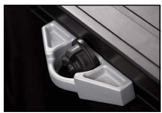
**Bed Cleat**—Add functionality with additional Bed Cleats. Designed specifically for the Tundra Bed Rails, they are constructed of sturdy die-cast aluminum, and each fully adjustable Bed Cleat is rated for a maximum load of 220 lb. Sold individually.
