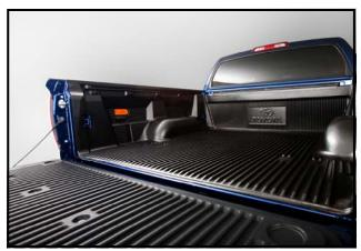
**Bed Liner**—Keeping Tundra's bed looking new; the custom-fitted Bed Liner for Tundra not only protects against dents and scratches but also reduces mold and mildew by allowing drainage and increased airflow. The Liner, featuring a nodrill attachment system and made from highdensity polyethylene copolymer, keeps loads from moving around in the bed. The Bed Liner also includes protection for the tailgate.
