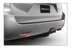
Hitch, Ball Platform and Wiring Harness - 1 1/4 inch Receiver
