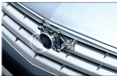
Radar-based adaptive cruise control sensor
