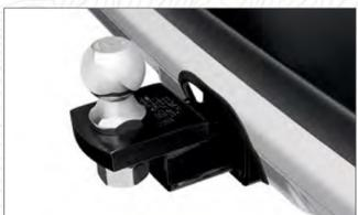
**Trailer Hitch.** Heavy-duty 2-inch receiver rated at 3,500 lbs. towing capacity, 350 lbs. tongue weight for the 2.4L Turbo XT and Outback Wilderness models, and 2,700 lbs. towing capacity, 270 lbs. tongue weight for the naturally aspirated 2.5L.
