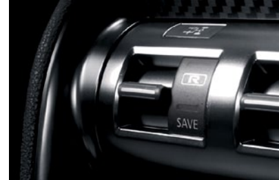
Transmission settings: R-Mode, Normal and Save
