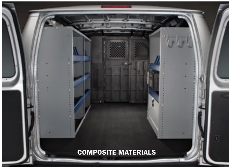
COMPOSITE SHELVING AND STORAGE REDUCES NOISE AND HELPS INCREASE FUEL EFFICIENCY
