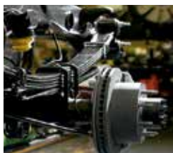
Asymmetrical rear suspension leaf springs.
