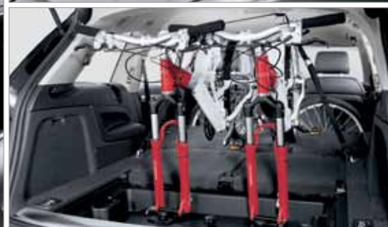
Aluminum bike rack 5 This locking holder fits 20- to 80-mm bike frames with both wheels on the bike and helps keep the bike upright as you secure it in place.
