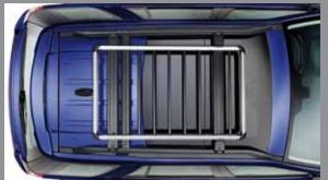
Load capacity: 125.66 lbs (57kg) on Roof Rails and Cross Bar.
