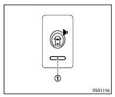
The warning systems switch will turn on and off the Lane Departure Warning (LDW) system and the Forward Collision Warning (FCW) system at the same time.
