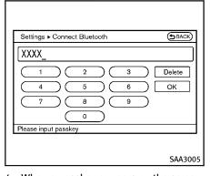
4. When a passkey appears on the screen, operate the compatible Bluetooth® audio device to enter the passkey. The pairing procedure for the audio device varies according to each audio device. See the Bluetooth® audio Owner's Manual for details. When pairing is completed, the screen will return to the Bluetooth® setup display.
