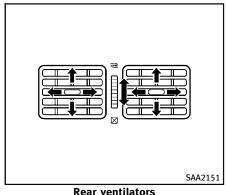
Open or close, and adjust the air flow direction of ventilators.
