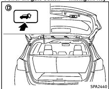
Power lift gate switch - Lift gate
