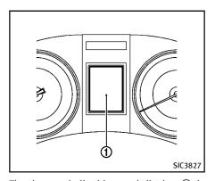
The dot matrix liquid crystal display (1) is located between the tachometer and the speedometer, and it displays the automatic transmission position indicator, the Intelligent Cruise Control (ICC) system (if so equipped), the Distance Control Assist (DCA) system (if so equipped) information, the Intelligent Key operation information and other warnings and information.
