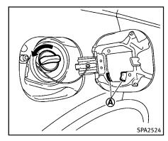
To remove the fuel-filler cap:
