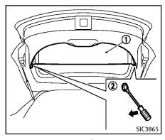
The rear cargo cover ① can be removed from the lift gate.
