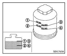
Check the fluid level in the reservoir.
