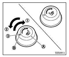
The front seats are warmed by built-in heaters. The switches located on the center console can be operated independently of each other.
