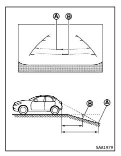
is the place (B). Note that any object on the hill is closer than it appears on the monitor.
