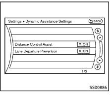
3. To set the LDP system to on or off, highlight the "Lane Departure Prevention" key, select ON or OFF and push the ENTER (2) button.
