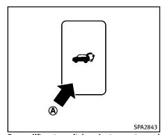
Power lift gate switch — Instrument panel
