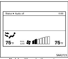
You can individually set the driver and front passenger side temperature using each temperature control button.
