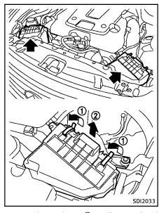
Remove the retainers (1) as illustrated and pull out the filter element (2).
