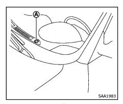
The sunload sensor (A) on the instrument panel helps maintain a constant temperature. Do not put anything on or around this sensor.
