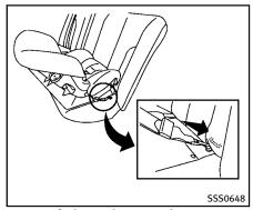
Rear-facing web-mounted — step 2 2. Secure the child restraint anchor attachments to the LATCH lower anchors. Check to make sure the LATCH attachment is properly attached to the lower anchors.
