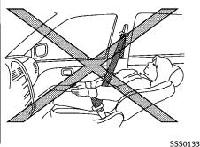
sits well back and straight up in the seat. If the seatback is reclined, the risk of sliding under the lap belt and being injured is increased.
