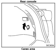
The power outlet is used for powering electrical accessories such as cellular telephones.
