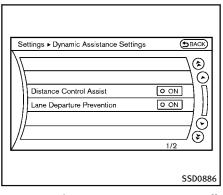
3. To set the DCA system to on or off, highlight the "Distance Control Assist" key, select ON or OFF and push the ENTER (2) button.
