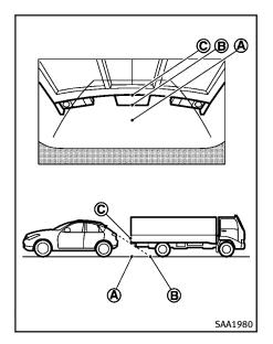
may hit the object when backing up to the position (A) if the object projects over the actual backing up course.
