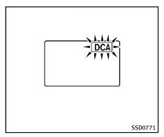
Under the following conditions, the Distance Control Assist system will not operate and the Distance Control Assist (DCA) system switch indicator light will blink:
