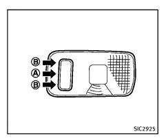
When the switch is in the DOOR position (A), the light illuminates while the lift gate is opened. When the lift gate is closed, the light will turn off.
