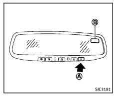
When the ignition switch is pushed to the ON position, the compass display (B) will indicate the direction of the vehicle's heading.
