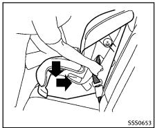
6. Remove any additional slack from the seat belt; press downward and rear-
