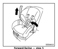
5. Allow the seat belt to retract. Pull up on the shoulder belt to remove any slack in the belt.
