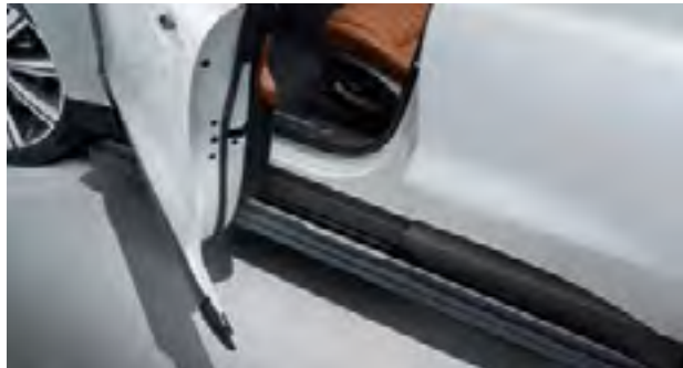
Electrically Deployable Side Steps* T4A12783 – Left Side T4A12780 – Right Side These smart, practical steps make it easier to get in and out of the vehicle and improve access to the roof. Neatly stowed under the sills, the side steps automatically deploy as soon as the door is opened. They stow automatically when the door is closed.
