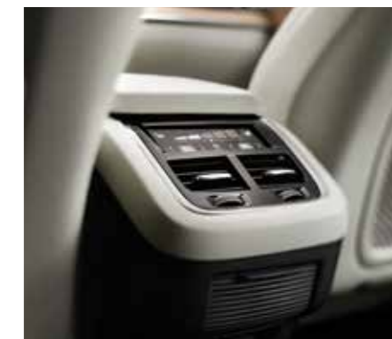
The four-zone climate system can be controlled from the center display touchscreen, or a graceful touch control panel at the end of the tunnel console.
